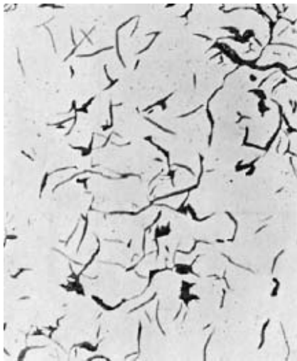
Fig. 6.3.2 Gray iron with flake graphite. Unetched, 100×.
